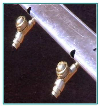
The **JARBA** Rotating Boom Assembly range has given the pilot control to adjust nozzle angles and boom lengths from the cockpit – delivering the correct droplet size at the right time.
