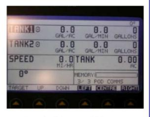
For in-flight variable rate control and mapping of liquids and dry material
